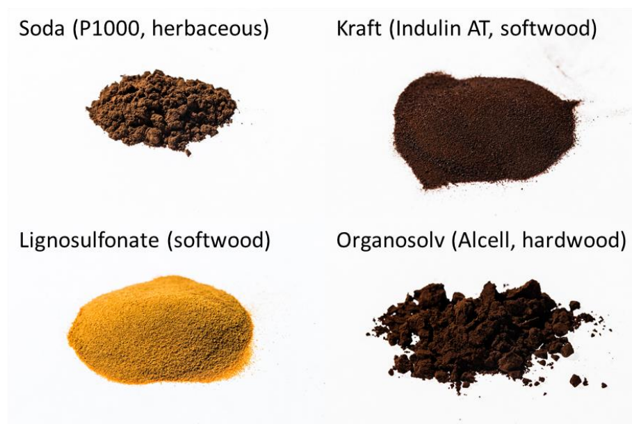
Figure 3. Photographs showing the differences in physical appearance for a number of typical technical lignins.
